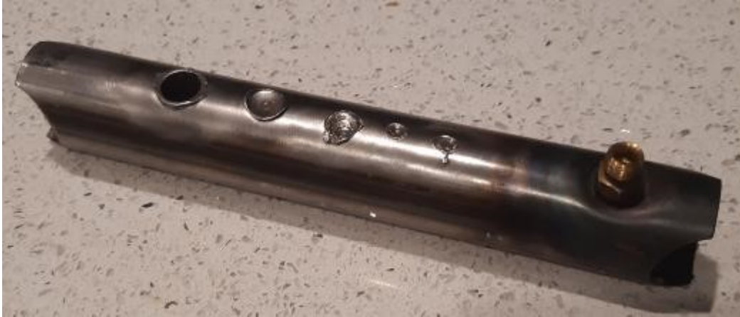
Mild steel ERW tube being test drilled to determine the best method of achieving a threaded hole in its 1.6mm wall thickness.
