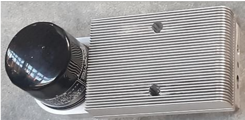
Combined oil filter and oil cooler machined in aluminium alloy.
