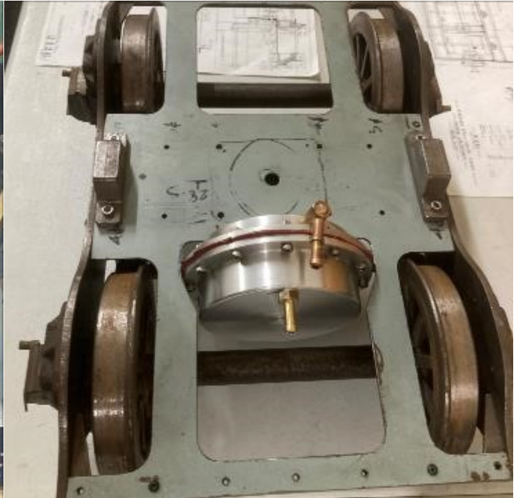
U class tender bogie with vacuum diaphragm fitted Photo Jon Mason
