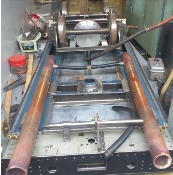
Vacuum braking setup being tested Photo Richard Lockett
