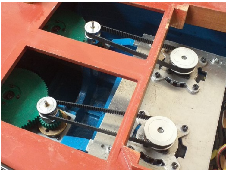
The drives to "Turihaua's" twin Azimuth Thrusters.
