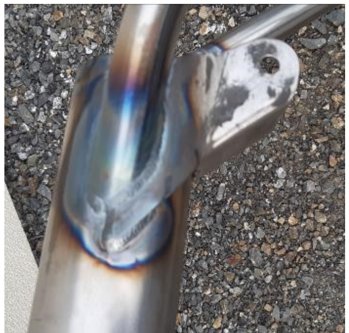
The top suspension mount nicely welded to the rear of the top tube.
