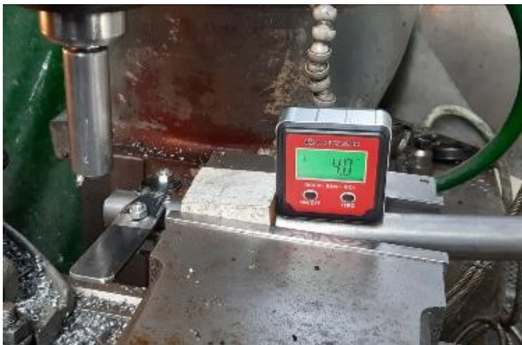
Tubes being notched using a fly cutter in a Milling Machine, digital angle gauge used to position tube.
