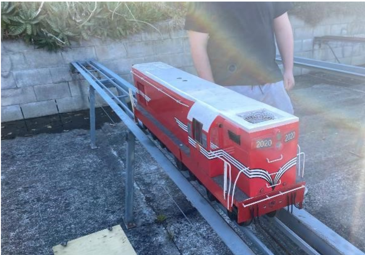
The first track run in April saw a visiting locomotive turn up, a 3.5 inch gauge NZR DA class owned by Jack Still and built by Grant Alexander up in the Waikato during the covid lockdowns. Powered by four 12 volt batteries and 24 volt motor from a battery lawnmower. One way of getting out of mowing the lawns I suppose. Photo Kyle Mudgeway
