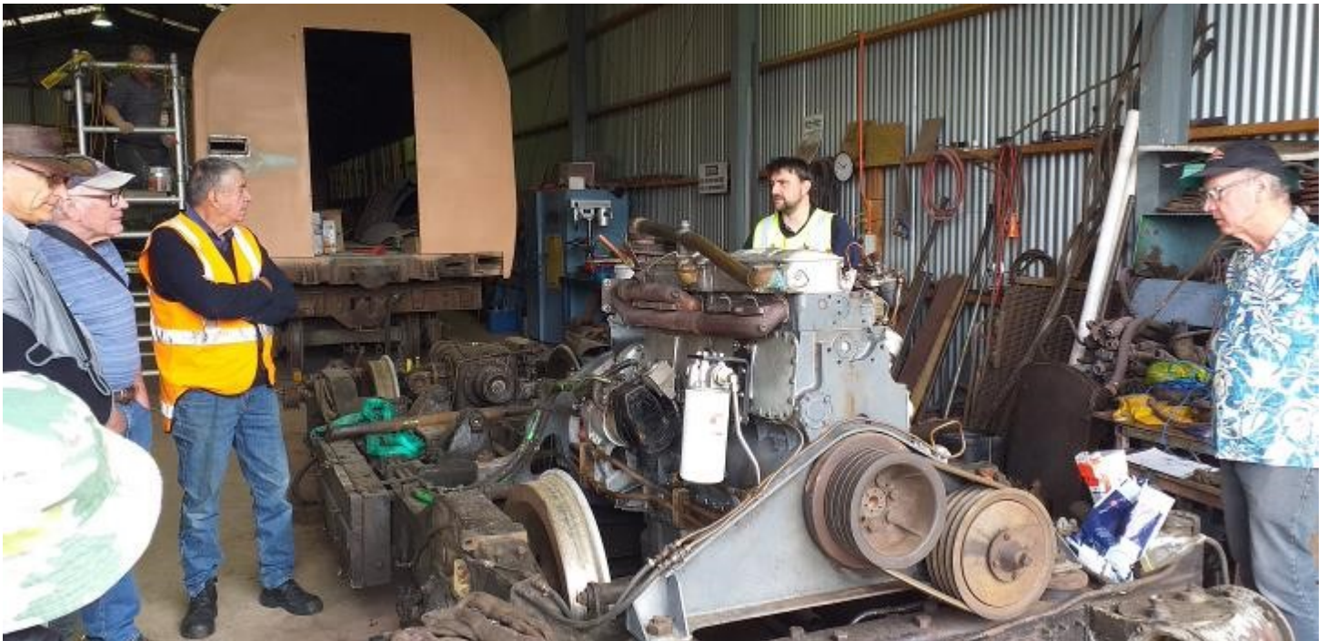
The 6 cylinder Leyland engine/transmission bogie from the PRS 1938 Standard Railcar out from under the frame to have a new head gasket fitted along with a host of smaller jobs while out.
