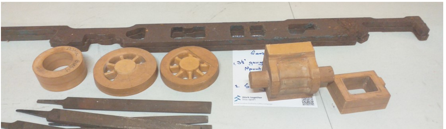
Frames and patterns for the Mountaineer in 3.5 inch gauge
