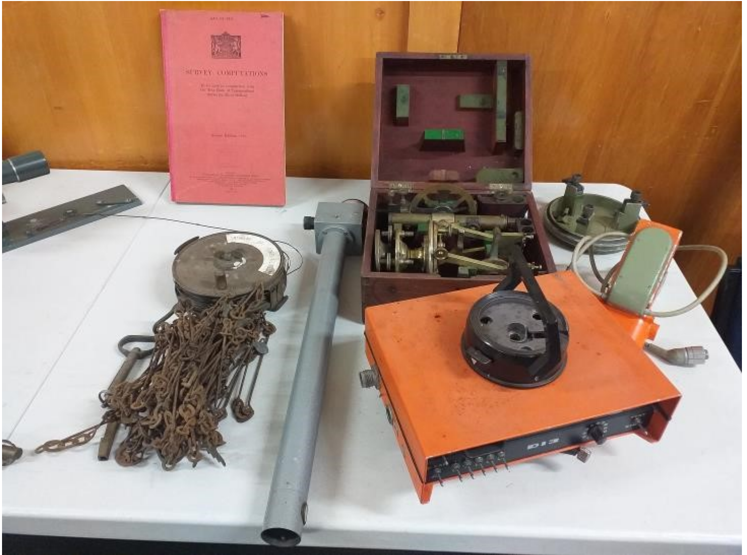
Gunter's Chain, a steel tape, very early theodolite in wooden case and the major upgrade to a light beam admitting orange box. Photo Editor
