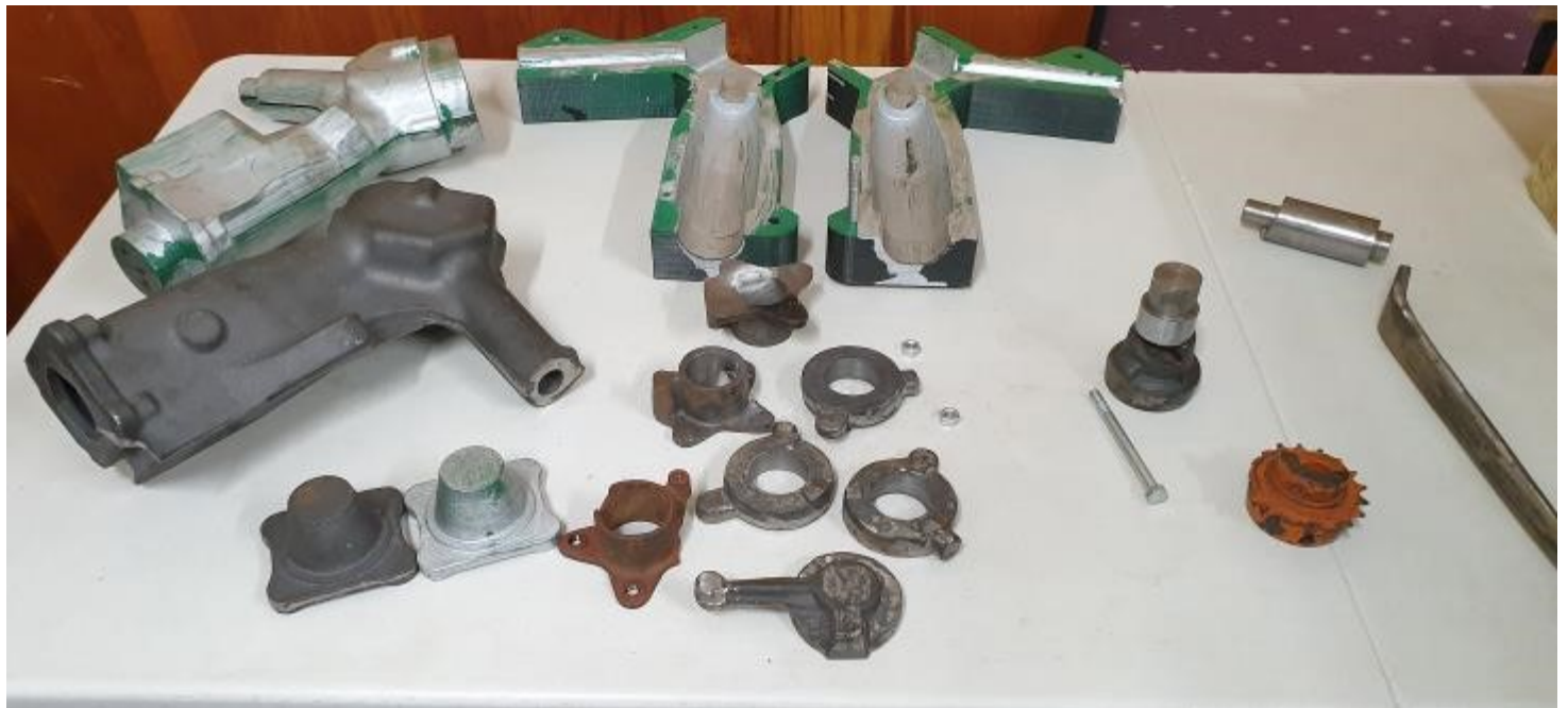
Cast Iron components for early Cadillac engines and the artillery piece part along with the 3D pattern and core box used in the casting process.
