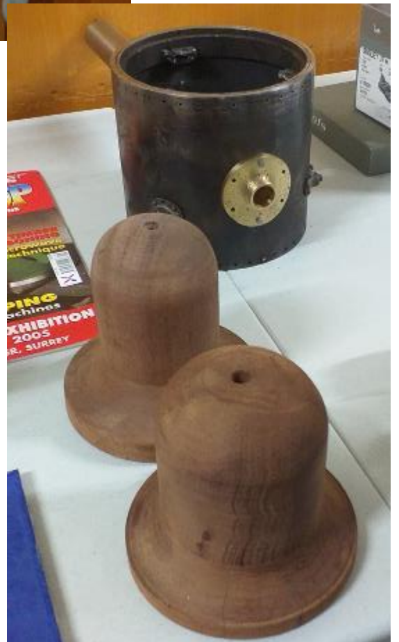
Sand and steam dome pattern's and smokebox for Ross Bridson's Shay locomotive. Ross wishes to form the domes out of sheet material rather than cast them.
