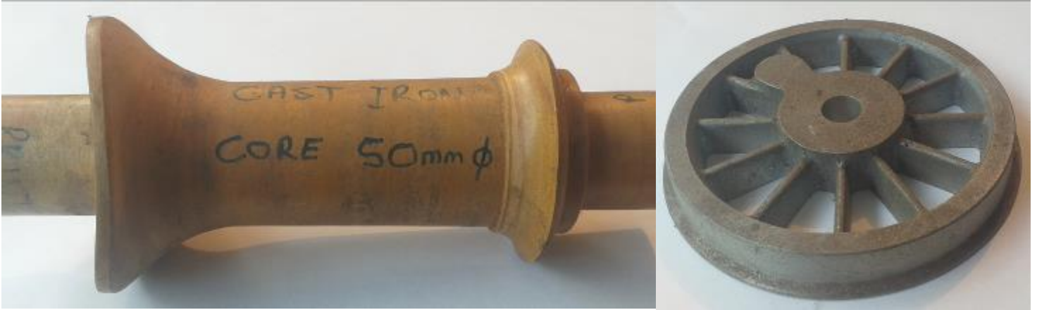
Pattern for a NZR steam locomotive chimney (W192) (S216) and cast iron wheel (W192)
