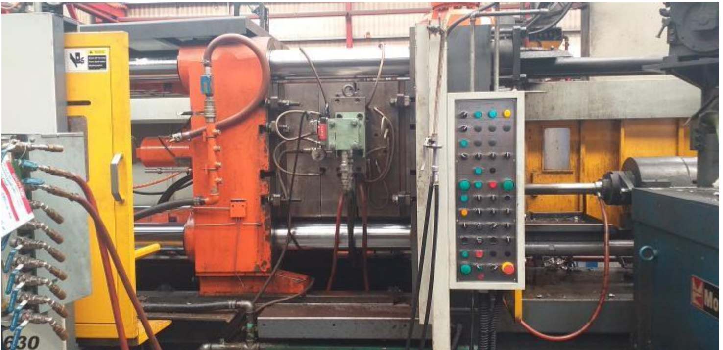
The moveable patten and closed die (centre) and shot tube (right) Photo Editor
