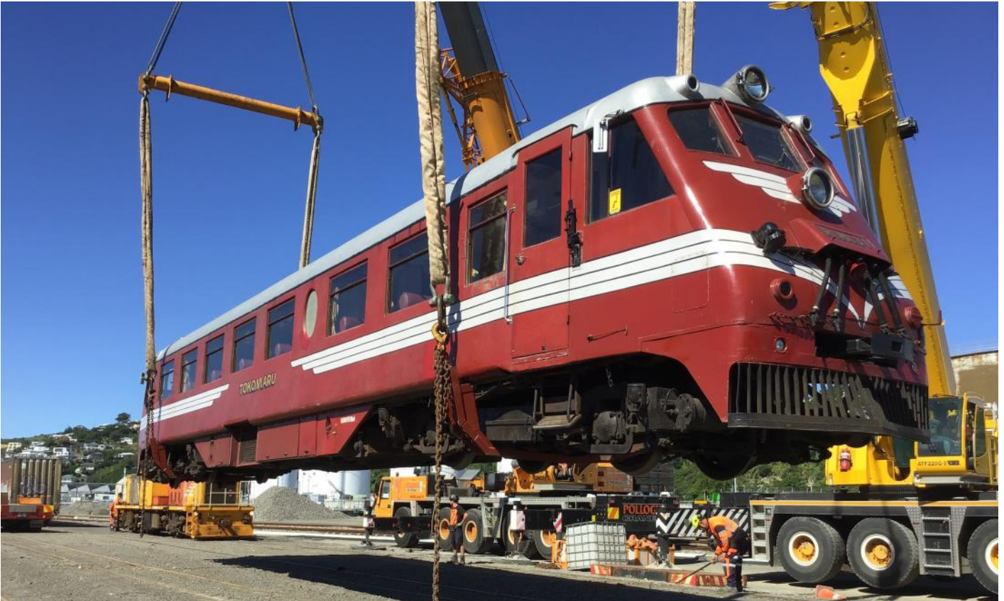
1938 Standard Railcar RM31 being lifted at the Napier Rail yards and about to be placed onto a Kenworth articulated low loader truck in preparation for a road trip back to Pahiatua.
