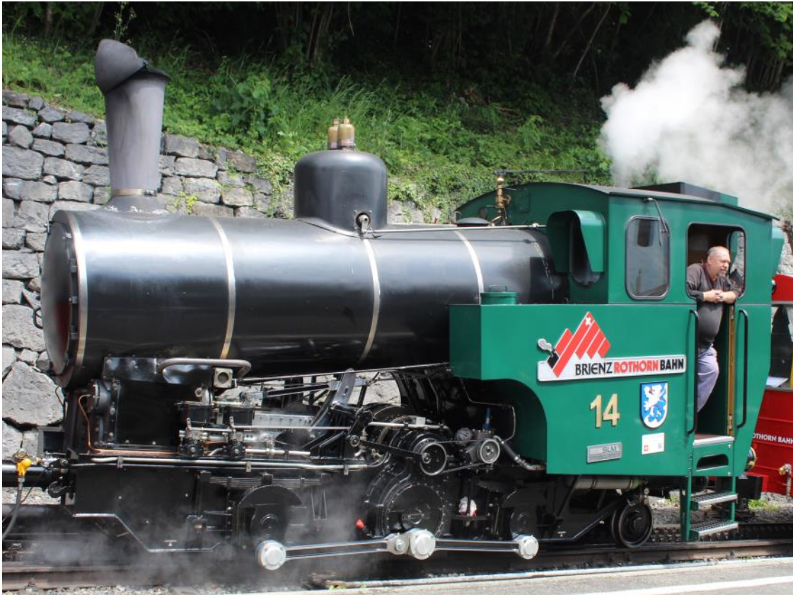
1996 oil burning Locomotive. Reduction gearbox located centre of driving frames.
