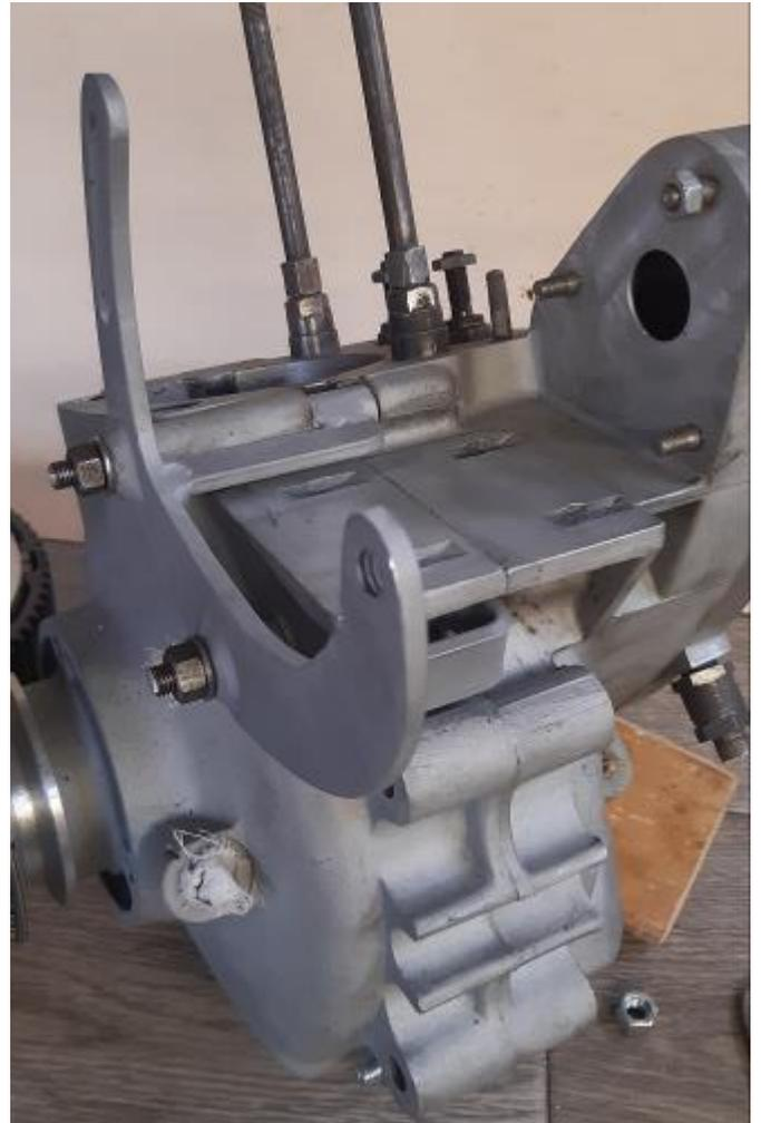
The finished alternator bracket fitted into place
