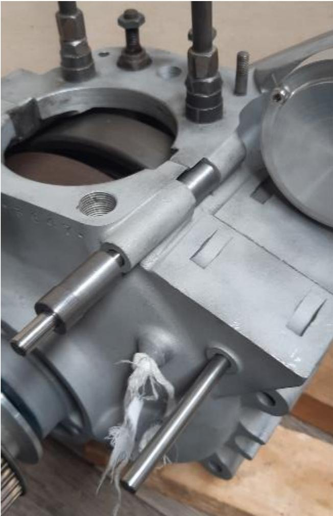
The new stainless steel studs and collars fitted up for mounting the alternator
