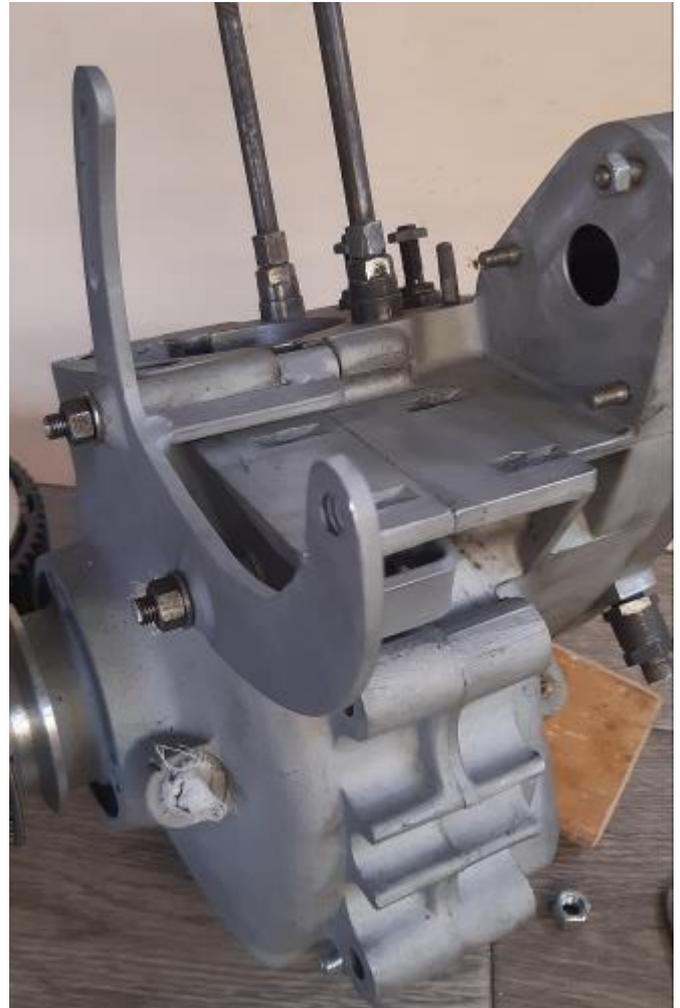
The finished alternator bracket fitted into place
