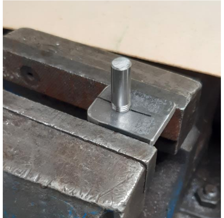
The clamp in use holding stud ready for threading.
