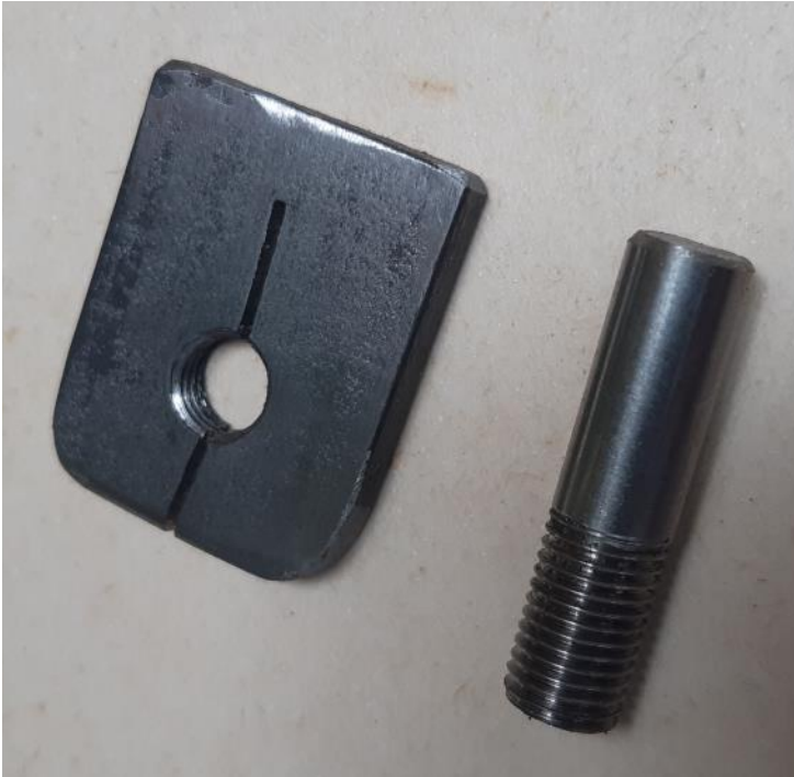
The threaded clamp and half completed stud.
