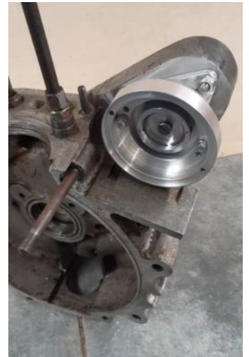
Left Timing case machined for custom housing.
