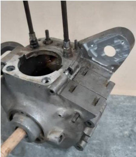
Left Timing case machined for custom housing.
