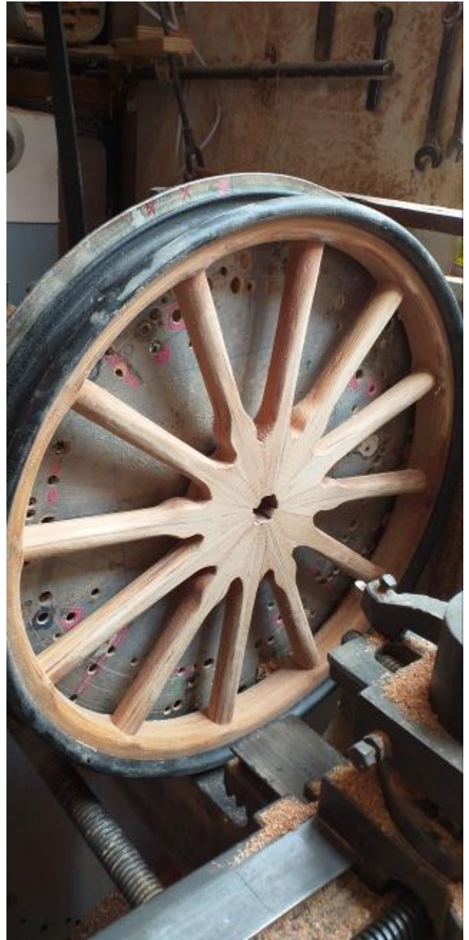
An assembled wheel mounted in a lathe for finishing machining of the bore and faces of the boss to accept the bearing caps.
