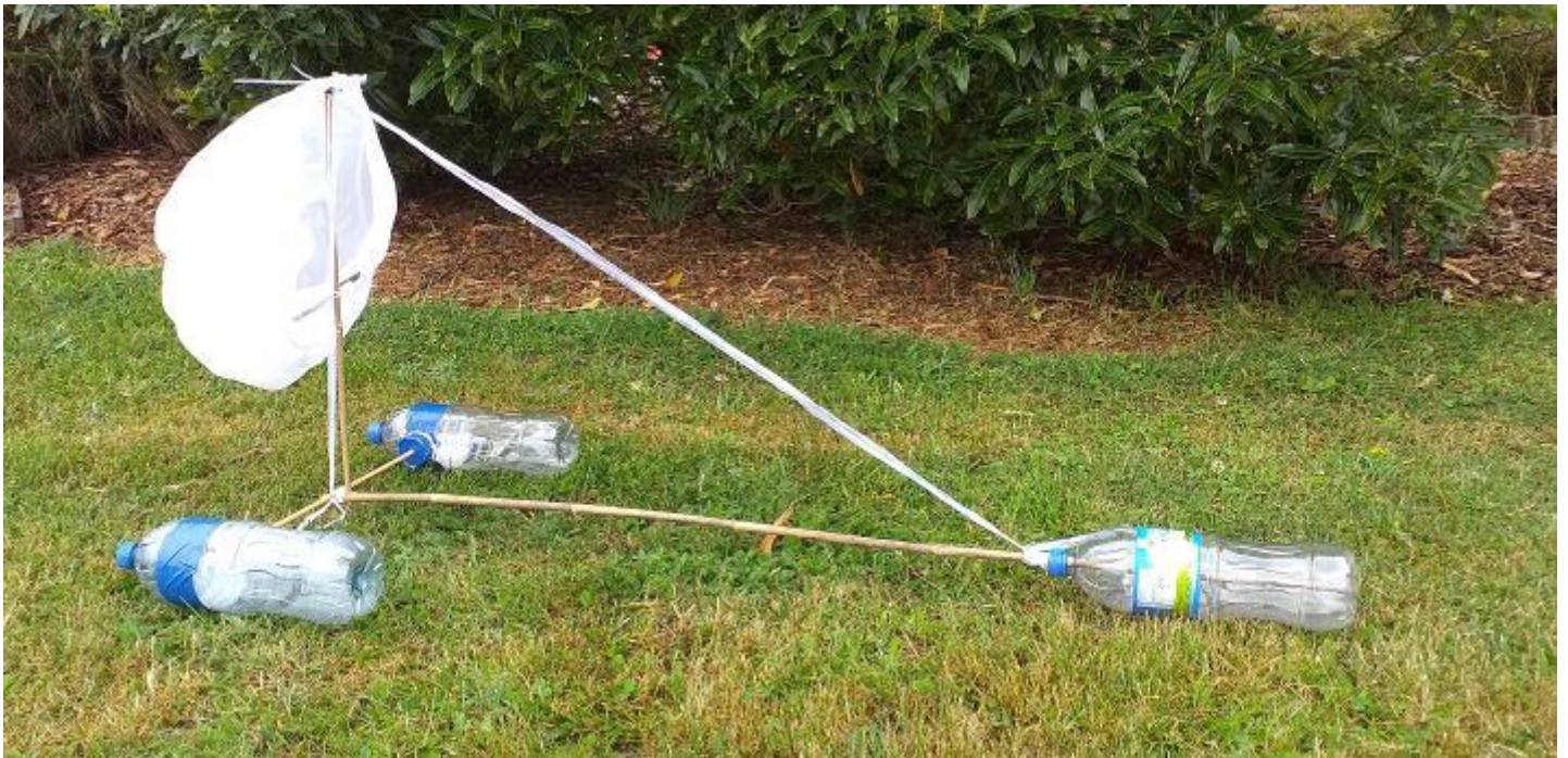
The PNMEC 2023 Les Moore Challenge Sail Boat awaiting the 3pm race start. Bamboo sticks, plastic drink bottles, cable ties, string and hot glue. Photo Editor
