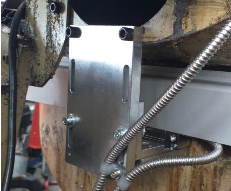
Mounting of Y axis scale and reader unit
