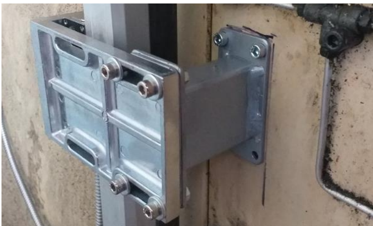
Additional bracket made for mounting of the Z axis reader.
