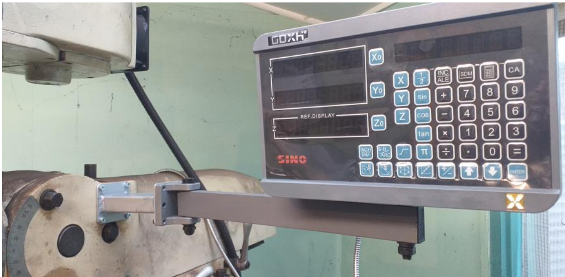
Additional bracket made to allow control unit to clear work lamp.
