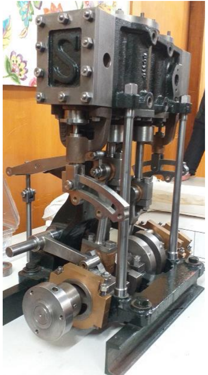
The Stuart Models 6A Compound Engine Photo Richard Lockett
