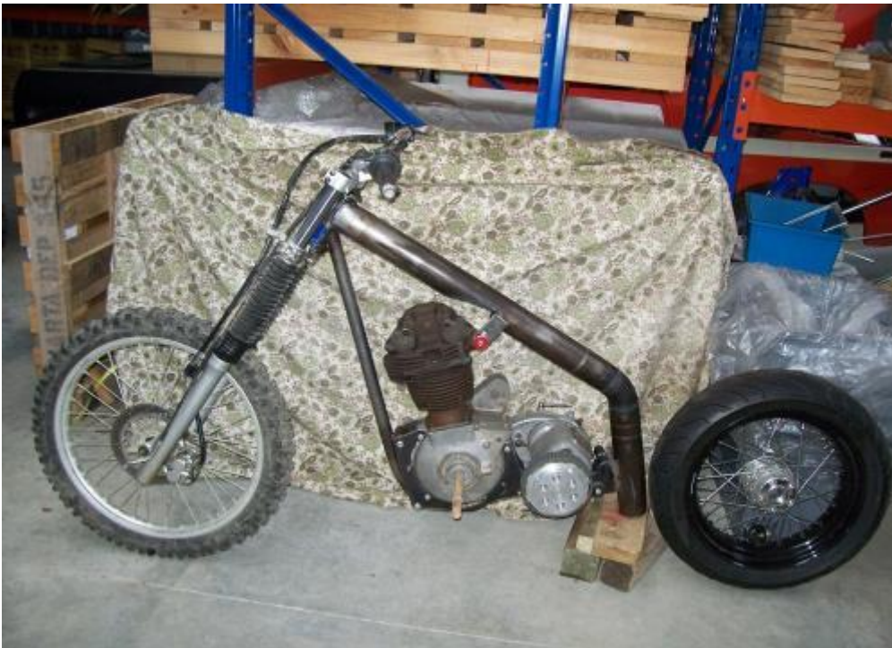
The Bobber, Yamaha forks, BSA 500cc motor with a custom frame.
