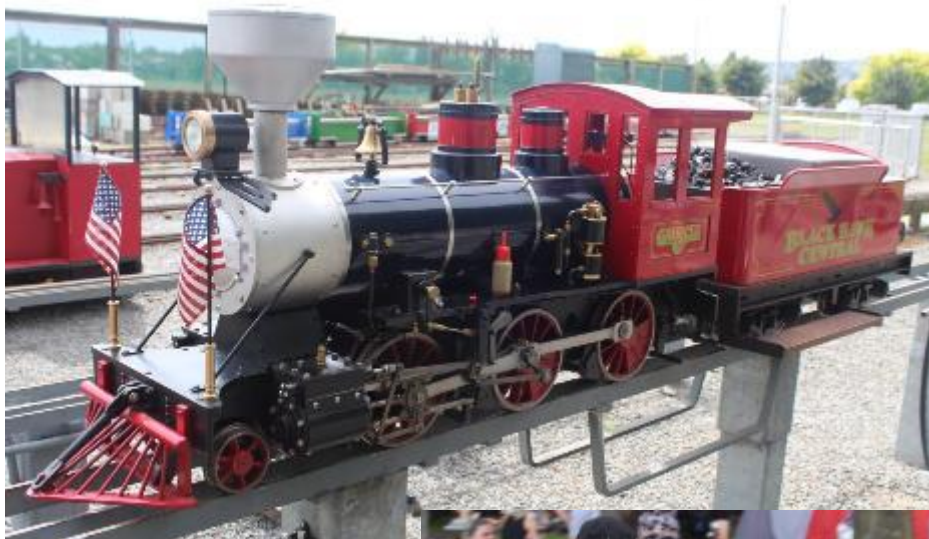
A nice example of the 7.25 inch gauge Phantom class 2-6-0 American style Locomotive designed by Manukau Live steamers Dave Giles of which dozens of examples have been built and are in operation around the world!
