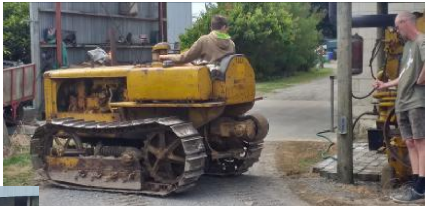
Kyle backing up the D2 crawler to act as the starter motor for the Caterpillar D397 engine.
