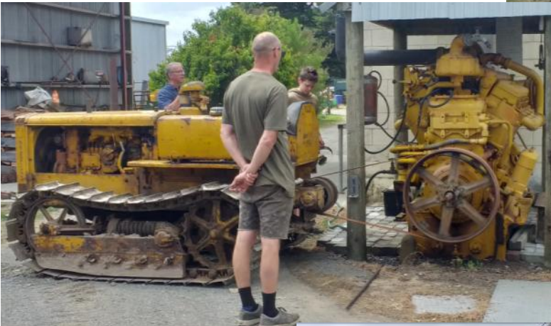
Starter Motor engaged the V12 turns over awaiting compression induced heat to ignite the diesel fuel and lift off!
