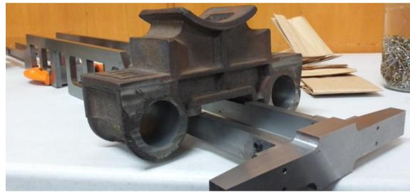
Frames and cylinder/ saddle casting for the 3.5" gauge 4-6-4 J series Hudson Locomotive.
