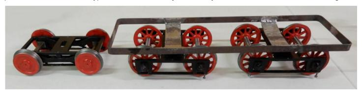
Ian McLellan brought along the tender frames, tender bogies, and leading bogie he has made for his "Virginia". Ian explained that the construction of this locomotive is a long term project but that progress is being made.
