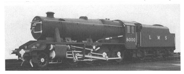
The above picture shows an LMS class 8F freight locomotive. This was the design ordered in 1939 by the War Department and used in France and elsewhere overseas. In 1943 the Ministry of Supply ordered further locomotives based on the Stanier 2 –8 –0 engines.
