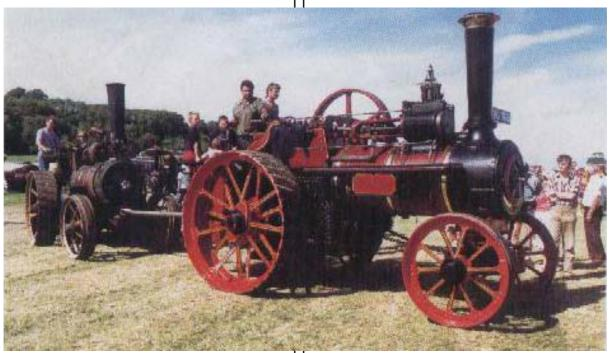
The Allchin was a four-shaft engine, crankshaft, second, third and axle and was sprung on both axles.
