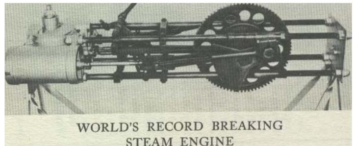
the stroke was 6 1/2". The piston were of the plain plug type, that is they had no piston rings, and the valve gear was Stephenson's. The engine turned 350 revolutions to the mile and the 34 inch diameter, 3 inch wide wheels turned 600 revolutions to the mile.
