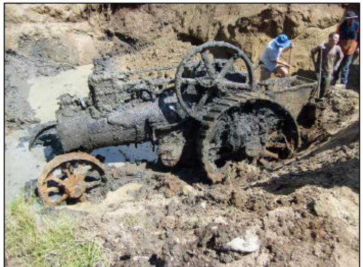
The steering wheel had been smashed, also the governor, chimney and chimney base which had all probably been smashed when the engine had been pushed into the creek. It was soon discovered that some off the controls, such as the cylinder drains, still moved freely. Much of the boiler cladding was
