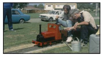
equally at home on a raised or ground level track. It could pull useful loads all day and had a free steaming boiler.
