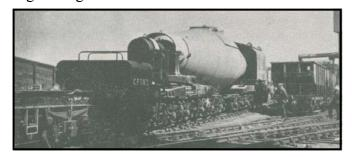
and North-West Durham. Each wagon carries 100 tons of molten metal and the total weight of each wagon when loaded is 241 tons, which is spread over 14 axles.
