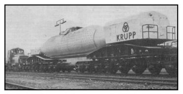
With a starting temperature of 1,400 C, the load only loses 5 C during the transit period. The container is emptied by rotating on its axis by electric motors in the end trucks. It takes just 4 minutes to empty the molten metal. In 1969 molten metal wagons were introduced in Britain. Three specially designed torpedo shaped
