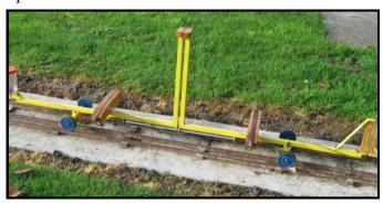
TTAFFY consists of two axles about 1.2 metres apart. One axle is attached to a steel tube and the other is attached to a bar which slides up into the tube. Each end has a level mounted near the axle and in the middle is a pair of pointers about 500mm above the frame. Each pointer is attached indirectly to the front or rear axle. These pointers greatly exaggerate the deflection between the two axles and the graduations on them are helpful in deciding the
