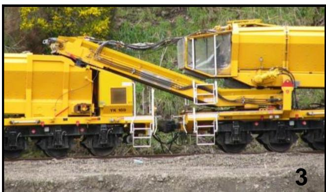
The third picture shows the details of the wagons. Each wagon has a sloped elevator in the floor and material can be moved along onto the next elevator which transfers the material onto the next wagon and so on until all the wagons are filled although the excavator has only been loading the wagon nearest the slip. Each wagon has an operator and a diesel engine powering a hydraulic pump which supplies oil to the oil motors that move the
