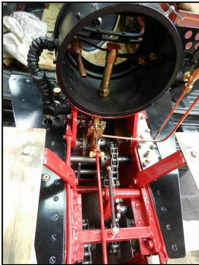
version of the original 1909 'Tesla' unit (rotor diameter only 65mm) easily fits between the frames.
