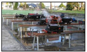
Four steamers on the steaming bays after a busy afternoon. It had been fine and sunny and there were a large number of passengers requesting rides. Three of the engines had had their fires dropped, boilers 'blown down' and were ready to be loaded into cars or vans. The nearest has still has wisps of steam drifting about and is soon to have its fire dropped and boiler blown down.
