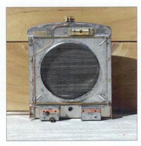
Front and rear views of the radiator and below the radiator fitted on the tractor. The radiator was constructed from tinplate with some brass components. 10 - 10BA bolts hold the radiator onto the tractor.
