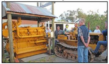
its own, the V12 was started using a flat belt driven off the power take-off on a D2 and once running the V12 had a real bellow combined with the whistle of the turbo charger.
