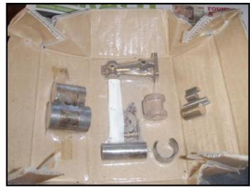
Steam Boiler feed pump \$50 Sets contain castings, bar stock and bolts etc all still in blister packaging.
