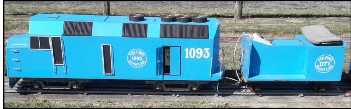
1093 a look-a-like of a American "F40PH" passenger hauling loco. It was originally built in October 1993, hence the number "1093" It has a "MyLocoSound" unit and 12 watt amplifier installed. 2 x120Ah Deep cycle batteries installed. Comes with 24v 8A charger. 4x 250Watt traction motors (2 in each Bogie).
