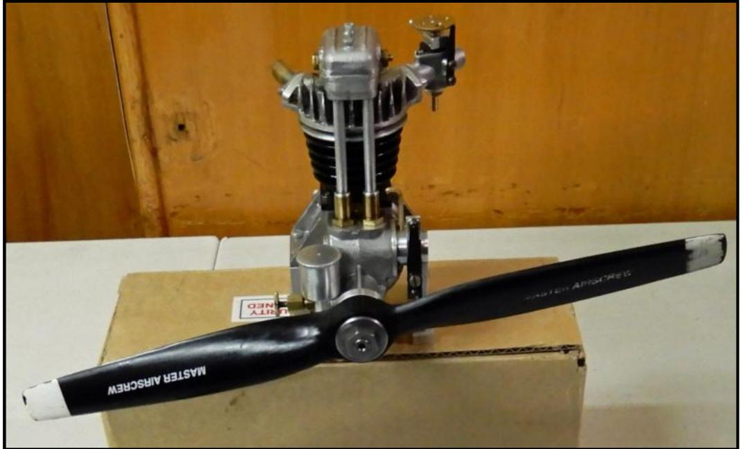
All parts were cleaned and on inspection revealed good quality die castings and most materials, including BA screws and nuts. Crankcase casting and cylinder head needed machining to correct dimensions – requiring a number of jigs and fixtures to be made.
