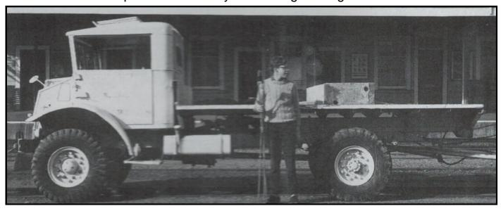
In operation the transporter was towed to the rail yards by the  $4 \times 4$ , with the faithful Prefect acting as pilot vehicle. Once located over the tracks the rear ramp was lowered and the wagon hauled up with the  $4 \times 4$ 's winch.
